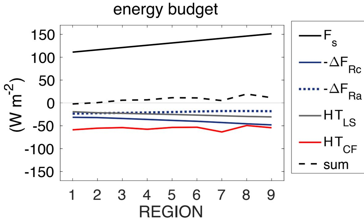
Fig. 13: Budget terms of the thermodynamic energy equation as a function of region (x direction). The fluxes are the surface flux (black solid), flux differences with minus sign due to longwave radiation in cloud cells (blue) and outside the cell region (blue dashed), divergence due to large-scale subsidence (gray), horizontal advection by background wind (red), and the residual (black dashed).
