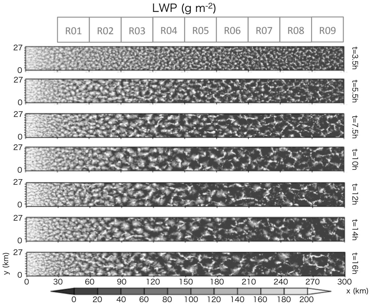
Fig. 1: Horizontal cross-sections of liquid water path (LWP,  $\text{g m}^{-2}$ ) at 7 selected timesteps. The abscissa and ordinate represent the streamwise and spanwise directions, respectively, and the units are kilometers.
