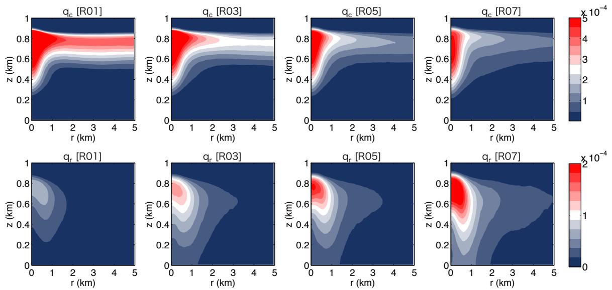
Fig. 8: Radius--height sections of the mixing ratio of (top) cloud water and (bottom) rain water for R01, R03, R05, and R07, which are composites of all samples from the cloud cells. Units:  $\text{kg kg}^{-1}$ .
