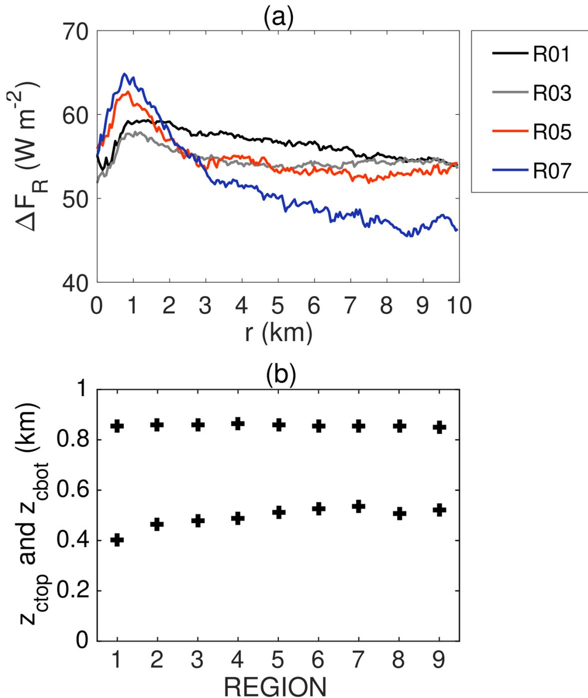
Fig. 10: (a) Radial profiles of vertical difference in radiation flux  $\Delta F_R$  averaged in the detected cloud cells. The black, gray, red, and blue lines represent R01, R03, R05, and R07, respectively. (b) Levels of cloud top and bottom, which are defined as  $q_t > 0.05 \text{ g kg}^{-1}$ , averaged in each subdomain.
