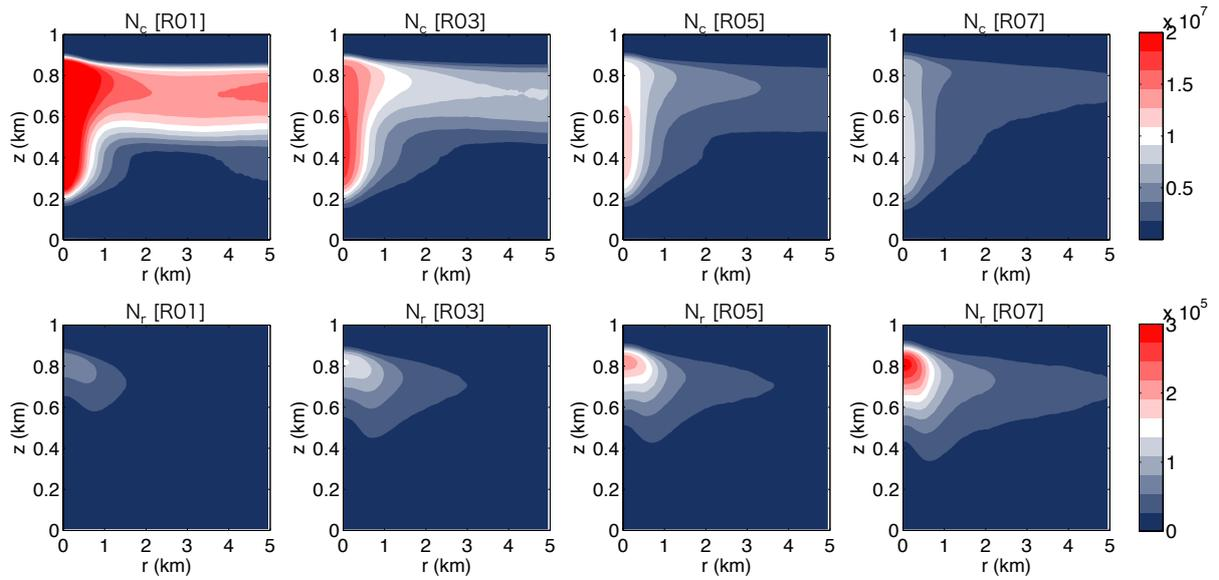
Fig. 9: Radius--height sections of the number density of (top) cloud water and (bottom) rain water for R01, R03, R05, and R07, which are composites of all samples from the cloud cells.
