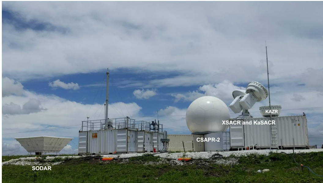
Fig. 2: ARM mobile facility deployed during CACTI-RELAMPAGO. Sensors left to right: Sonic Detection and Ranging wind profiler (SODAR), C-band Scan Precipitation Radar 2 (CSAPR-2), X and Ka band Scan ARM Cloud Radars (XSACR and KaSACR), and Ka-band Zenith Radar (KAZR).
