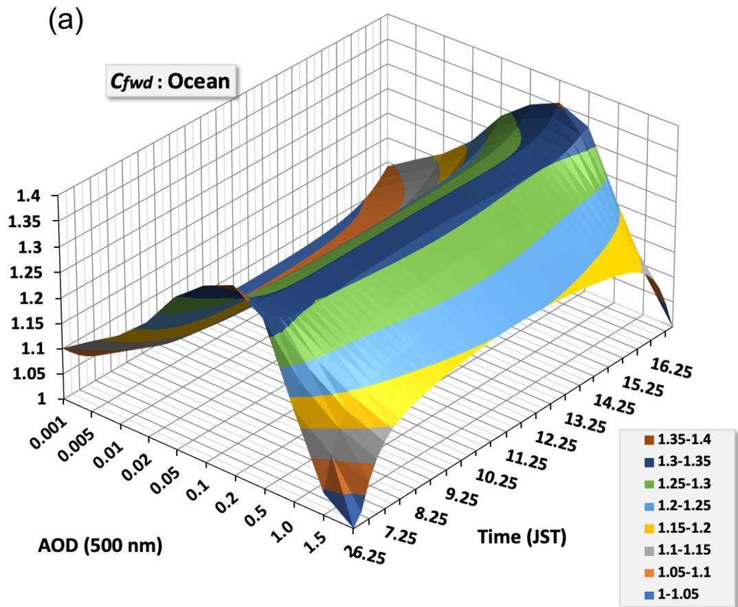
Fig. 6a Variation of the correction coefficient  $C_{fwd}$  as a function of AOD and time.
