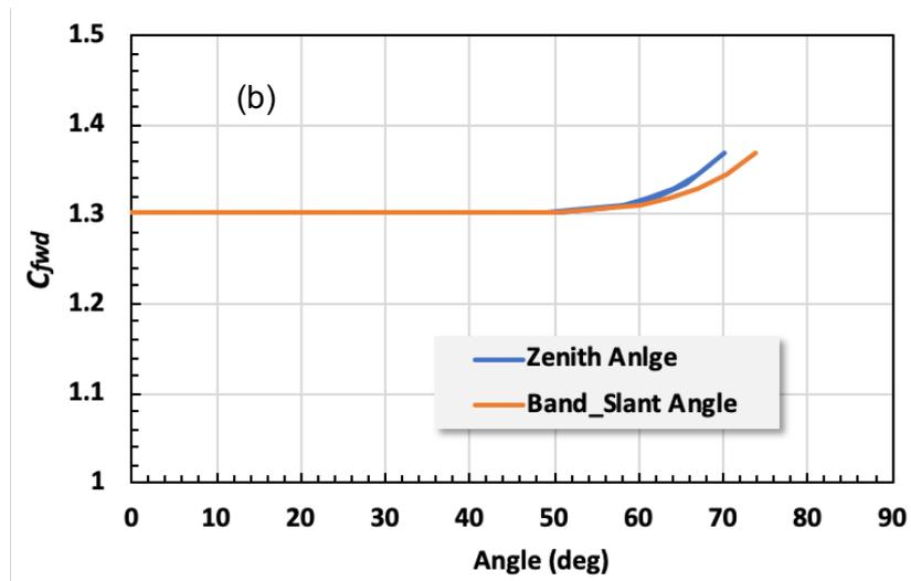
Fig. 5b Correction coefficient  $C_{fwd}$  defined by  $\Delta F_3 / \Delta F_{mean}$  as a function of the solar zenith and band slant angles. Curves are plotted with a fundamental error of less than 2%.
