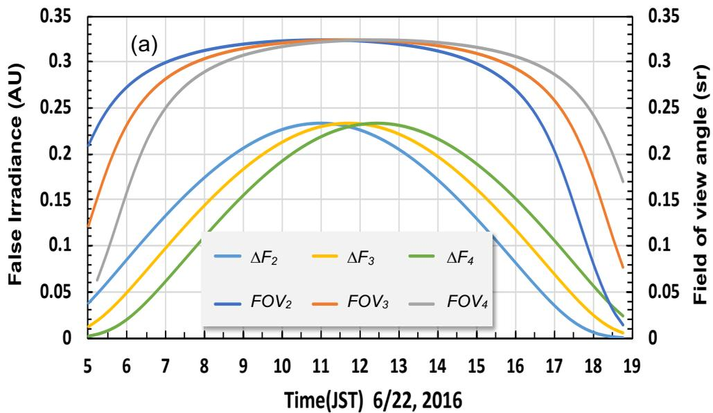
Fig.3a Time series for each band, of the field-of-view angle ( $FOV$ ), represented by the upper three solid curves and, the virtual radiation ( $\Delta F$ ) incident into a region shadowed by the band, represented by the lower three curves. The incident radiation is assumed to be unity, so these curves mean variations combined with the cosine characteristic and field view angle.
