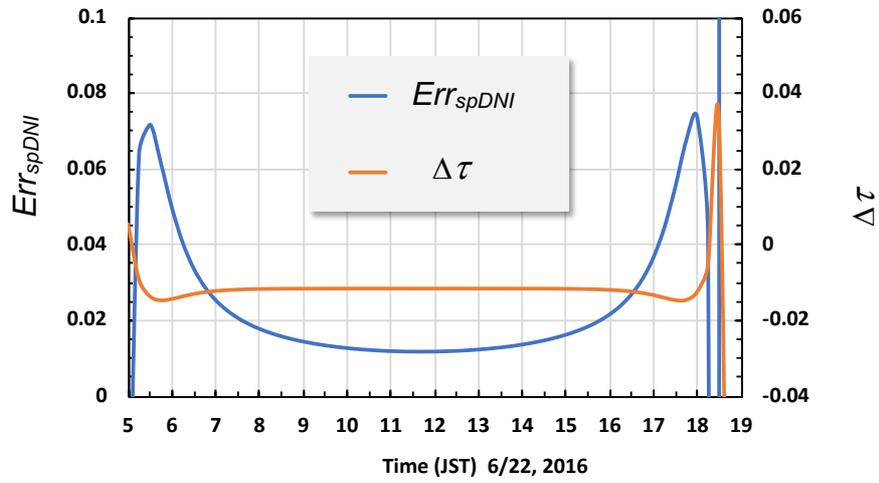
Fig. 7 An example of diurnal variation of relative error ( $Err_{spDNI}$ ) in spDNI and optical depth error ( $\Delta\tau$ ), defined by Eqs. 10 and 12. These are plotted for the Oceanic aerosol type with AOD of 0.2.
