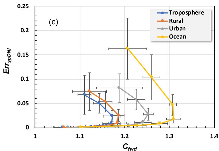
Fig. 8c Relative error in spDNI as a function of  $C_{fwd}$ . Seven AODs are used as the same in Fig.8a for each aerosol type. The upper ends of each line are for AOD=1.5. The error bars are the same as in Fig.8a.
