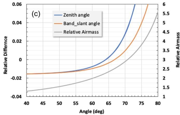
Fig. 3c Relative difference between the expected irradiance and the mean irradiance approximated by  $\Delta F_2$  and  $\Delta F_4$ , as functions of the solar zenith and band slant angles. For less than 72 deg band slant angle, the fundamental error due to the cosine characteristic including the band geometry is about less than 2%. The relative airmass corresponding to the solar zenith angle is plotted as a reference.
