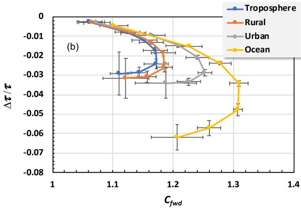
Fig. 9b Estimation error in optical depth as a function of  $C_{fwd}$ . The four lines with error bars indicate different aerosol types for seven AODs, 0.01, 0.05, 0.1, 0.2, 0.5, 1.0 and 1.5. The lowest ends of each line are for AOD=1.5, and the smallest (upper) points are for AOD=0.01.
