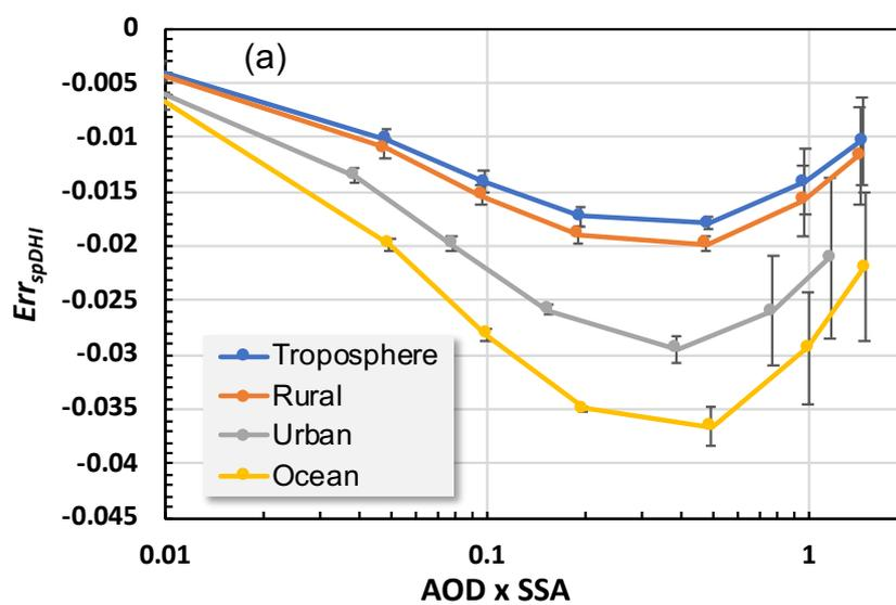
Fig. 11a Relative error in spDHI estimation as a function of AOD x SSA. Each aerosol type shows the minimum points during a range of 0.1 to 1.0 AOD x SSA.
