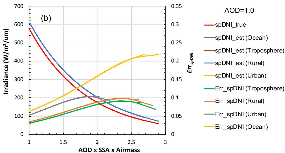
Fig. 8b Examples of spDNI and  $Err_{spDNI}$  as a function of AOD x SSA x Airmass for four aerosol types with AOD of 1.0. The estimated spDNIs (spDNI\_est) for each aerosol type overlap on the same lines due to small differences. The patterns of  $Err_{spDNI}$  show peaks depending on the aerosol type.
