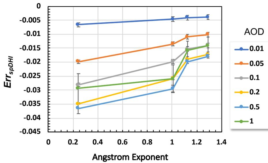
Fig. 12 Relative error in spDHI estimation as a function of the Angstrom Exponent (AE) with different AODs, ranging from 0.01 to 1.0. Four aerosol types are shown corresponding to their AEs.
