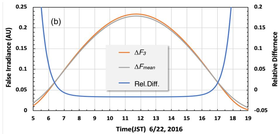
Fig.3b Time series of virtual radiation and the difference between the expected irradiance  $\Delta F_3$  (for isotropic radiation) and the mean irradiance approximated by both side ones ( $\Delta F_2$  and  $\Delta F_4$ ).
