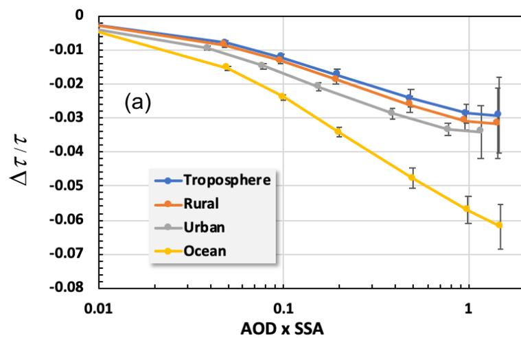
Fig. 9a Relative error in optical depth as a function of AOD x SSA. The four lines with error bars indicate different aerosol types for seven AODs, 0.01, 0.05, 0.1, 0.2, 0.5, 1.0 and 1.5. The rightmost ends of each line are for AOD=1.5.
