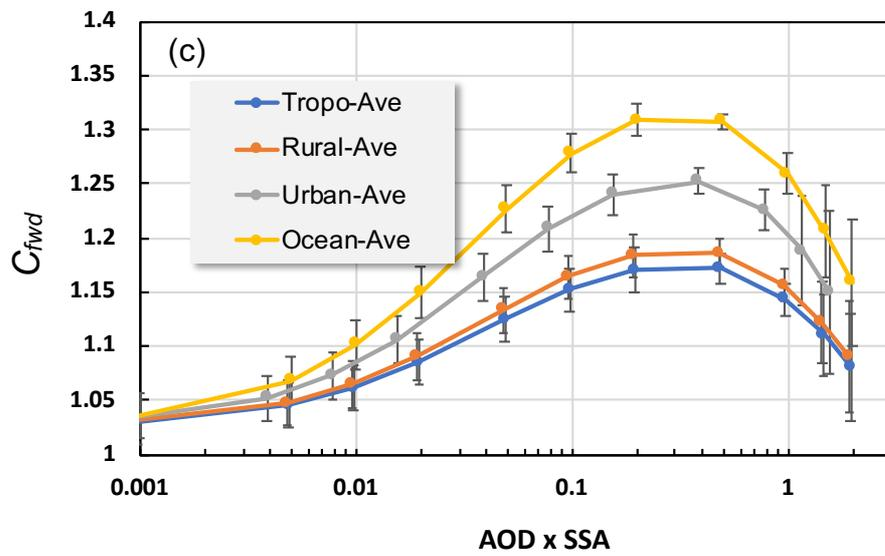
Fig. 6c Variation of mean correction coefficient  $C_{fwd}$  as a function of AOD x SSA.
