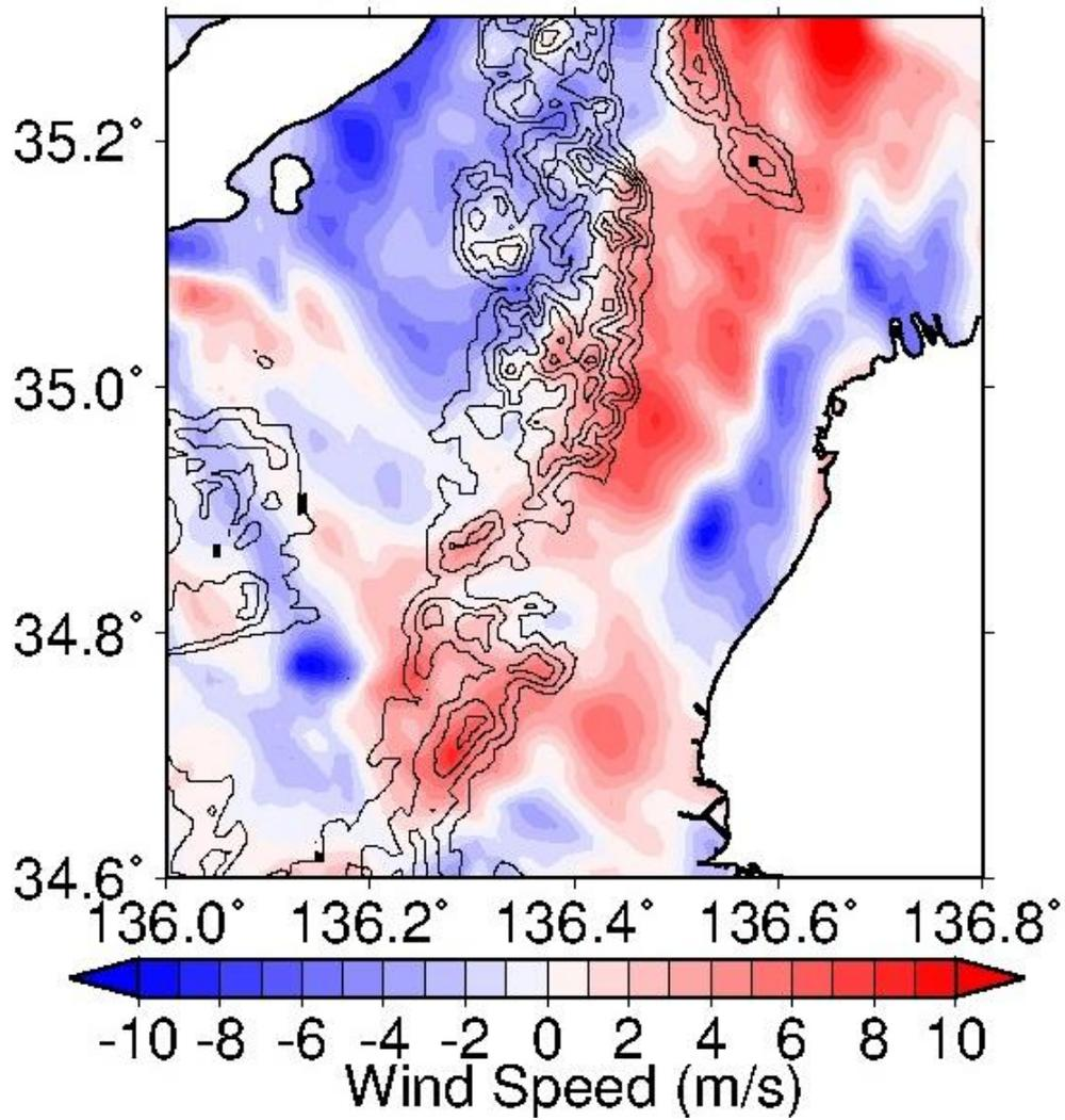
583 Fig. 12. Impacts of mountains on the surface wind speed (cases CTRL - NoMt) at 1700 on
