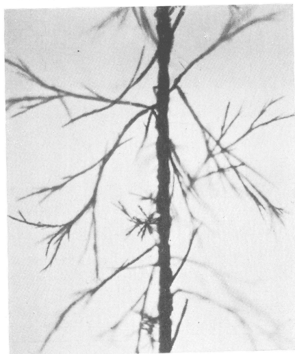
A peculiar type of crystals developed from a silk thread wetted with methyl silicone oil, DC 200, 100 c.s. T = -18^{\circ}\text{C} . \times 6.9
